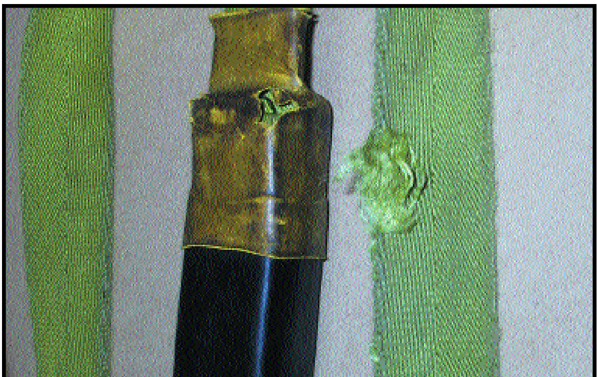
Damaged webbing and protector to energy absorber
