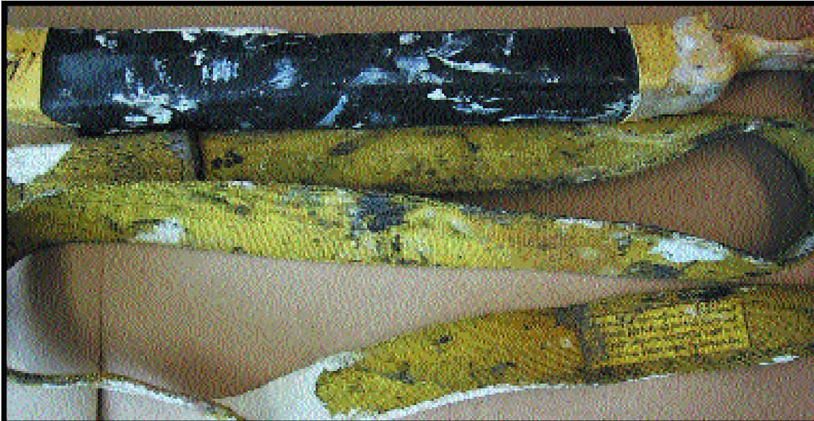
Heavy paint contamination to webbing
