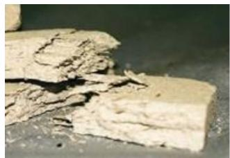
board (AIB) ceiling that formed a fire break between it and the rest of the house. During the conversion work between 8 May and 2 August 2012, the boards were removed, broken up and left on the homeowners' front lawn.
